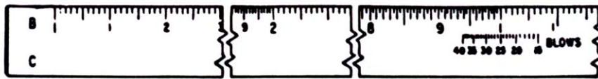
A - LOCATION OF SPECIAL SCALE (BLOWS) WITH RESPECT TO B SCALE OF SLIDE RULE
