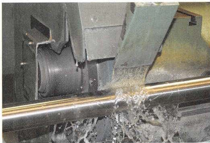
Figure 19-17. Coolant must flood the area being ground.
