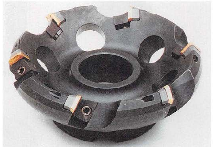
Figure 17-33. Face mill with indexable inserts. A—The replaceable inserts are mechanically clamped in place on the cutter body. As cutting edges wear, the inserts can be turned (indexed) to present a fresh cutting edge. B—An example of a face mill with indexable inserts. Insert selection is based on the material to be machined.
