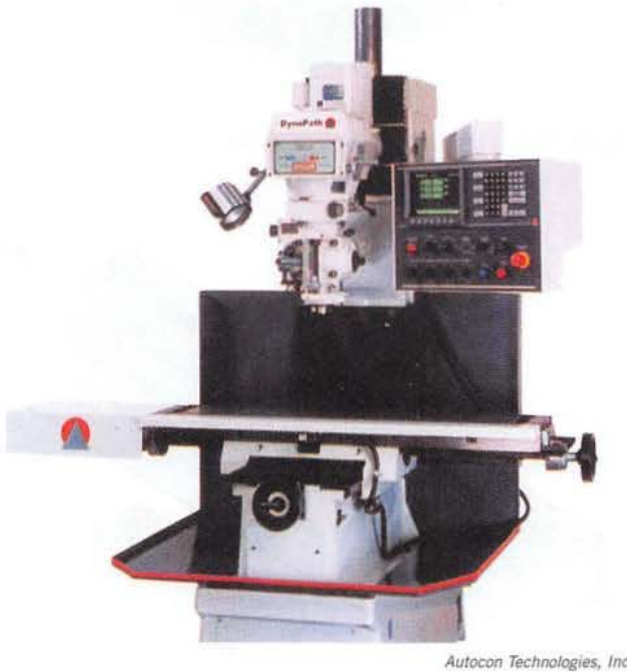
Figure 17-4. Fixed-bed or bed mills have a very rigid worktable that moves only in a longitudinal direction. The machine shown can be operated manually or by CNC.
