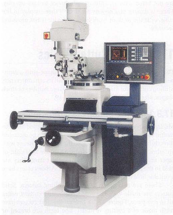
Figure 17-15. This manual vertical milling machine was retrofitted with a CNC control unit. The retrofit provides two-axis (X and Y) machine control capabilities and displays depth (Z axis) information on the monitor.
