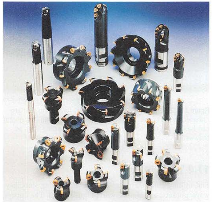
Figure 17-21. A variety of cutters with indexable carbide inserts. When the cutting edges dull, new cutting edges are rotated into position. The inserts are available in different grades. The grade chosen for a job depends on the material being machined.
