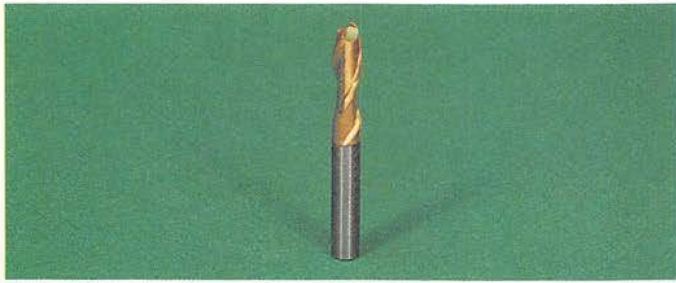
Figure 17-30. The two-flute end mill can be fed into work like a drill.
