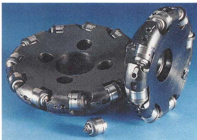
Figure 17-34. This face milling cutter has an unusual design, making use of bearing-mounted inserts that rotate as they cut. The manufacturer claims that the better heat dissipation provided by the rotating inserts increases cutter life and permits higher cutting speeds.
