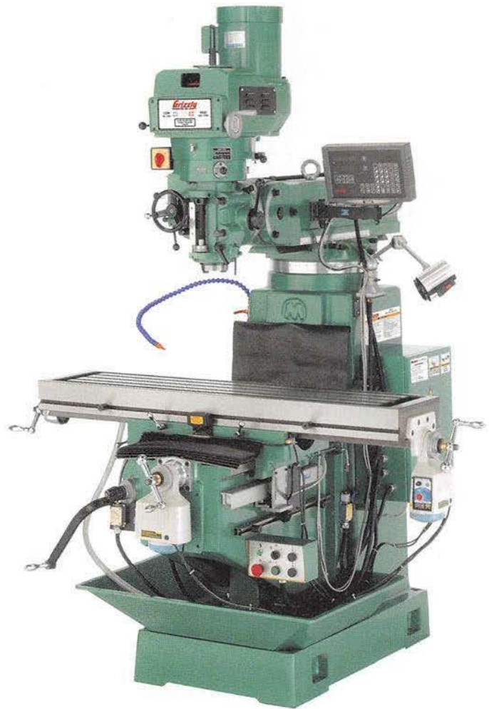
Figure 17-2. A knee-type vertical milling machine that incorporates longitudinal and traverse power feeds, digital readout, and a built-in coolant system.
