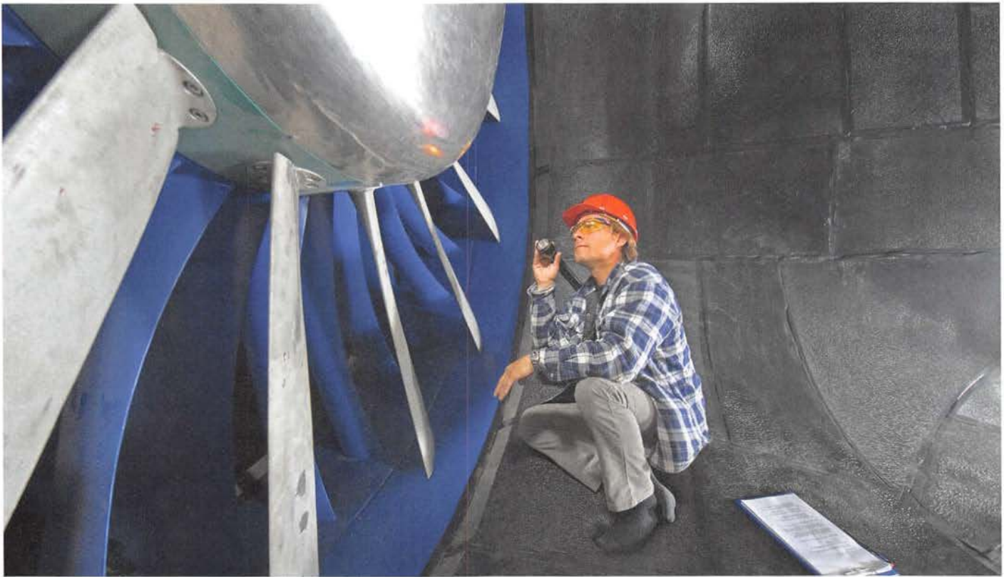
Figure 2-13. An engineer inspects the rotors of a huge industrial wind turbine that will be used to test the aerodynamic qualities of everything from aircraft to automobiles.
