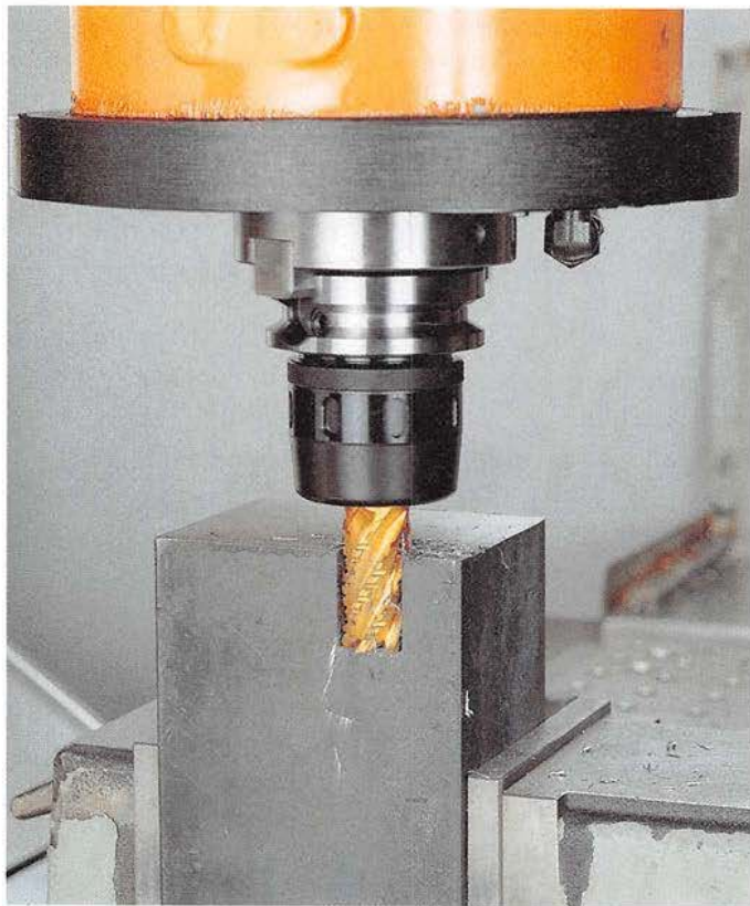
Figure 17-1. A milling machine rotates a multitoothed cutter into the workpiece.
