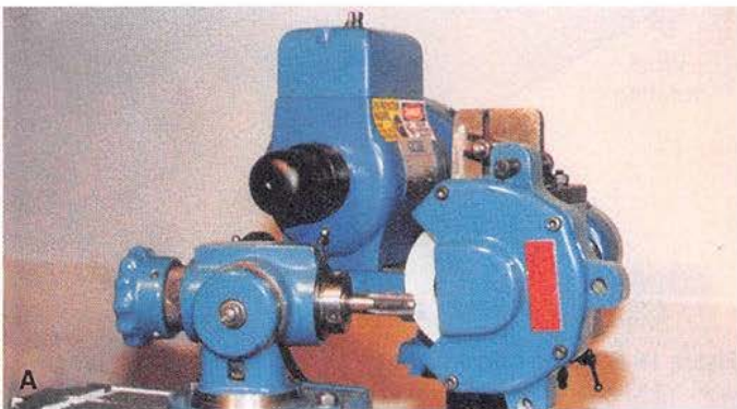
Figure 19-35. Grinding taps. A—Setup for regrounding a chamfer on a tap. B—Flutes are being reground on a tap to renew the cutting edges of the teeth.
