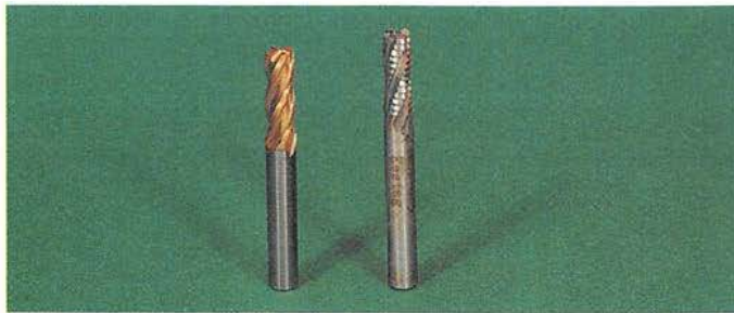
Figure 17-31. Multiflute end mills. The peripheral grooves in the cutter at right reduce chip size, lowering cutting forces. Most modern cutters have a nitride coating that improves resistance to abrasive wear and corrosion.
