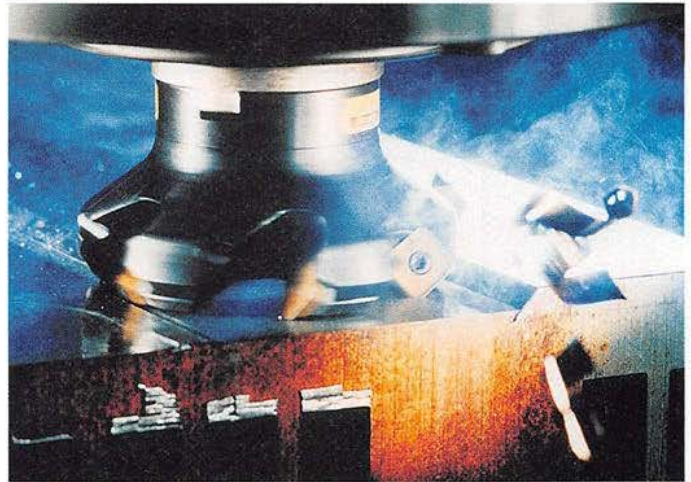
Figure 17-16. Face milling. A—The surface being machined is parallel with the cutter face. B—An example of face milling.
