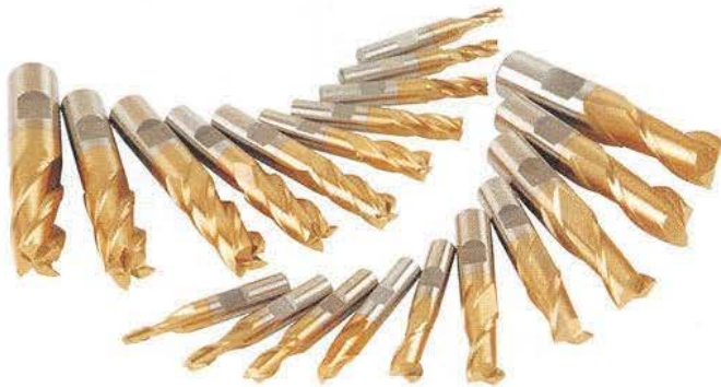
Figure 17-20. A selection of two- and four-flute HSS solid milling cutters. The gold on the cutters is a titanium nitride (TiN) coating that increases wear resistance and the lifetime of the cutter significantly.
