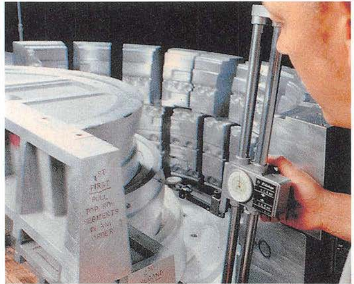
Figure 2-6. A tool and die maker checking the dies used for molding a plastic pattern used to cast a jet engine component. Master tooling ensures that other sections of the engine, made elsewhere in the United States, Israel, and Europe, will fit together perfectly.
