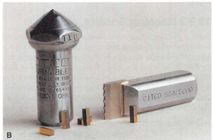
Figure 19-9. Diamond wheel dressing tools. A—Close-up of a natural diamond chip on a grinding wheel dresser. The diamond should be rotated a partial turn each time it is used to put a new edge of the diamond into position. B—Dressing tools manufactured from manmade diamonds. These diamonds do not have the irregularities of natural diamonds, resulting in consistent diamond exposure and longer wear.
