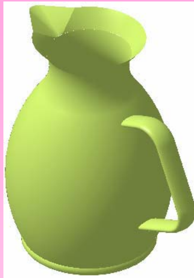
Figure L The isometric view of the model after splitting the swept surface
