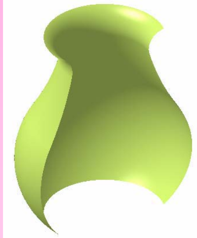
Surface revolved through an angle of 180-degree
