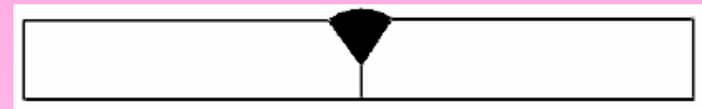
Drawing view after adding the welding symbol
