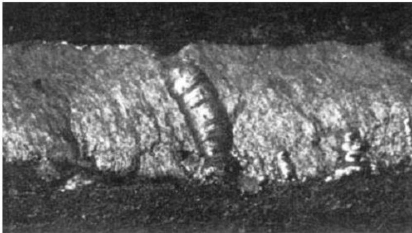
Figure 3.25 Wormhole porosity in weld metal. From Jackson (55).
