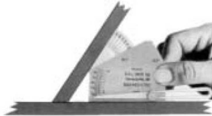
Checking Angle of Vertical Member
